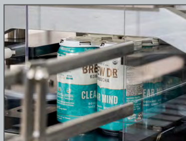
Applies Can Carriers in Dual Lane Format
