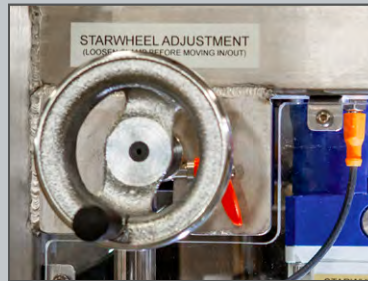
Simple Can Diameter Change
