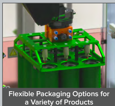
Two Independent Magazines per Robot
