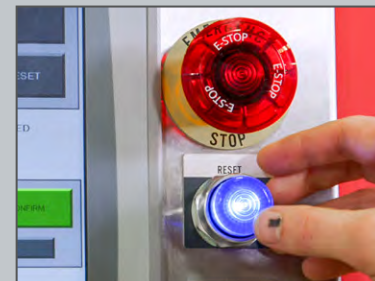
Category III-PLD Safety System
