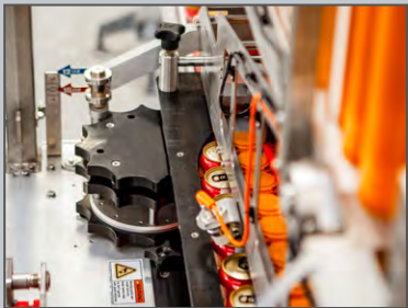
Servo Driven Starwheels
