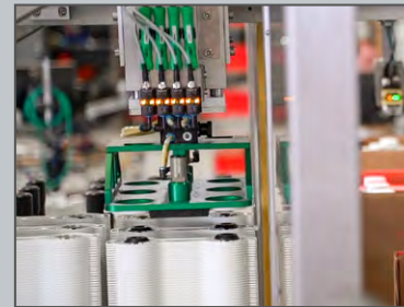
Automatic Handle Magazine Shuttle
