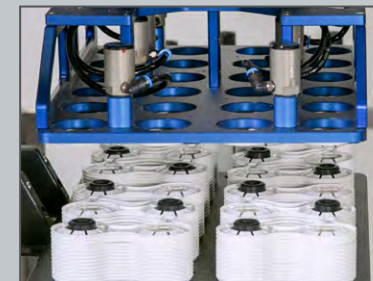
Dual Axis Pick and Place Layout
