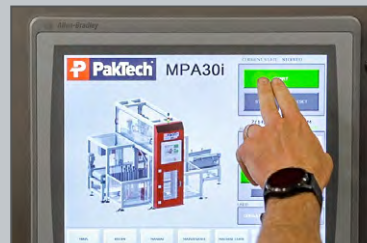
HMI Touch Screen, Status & Alarm Messaging & I/O Status Screens
